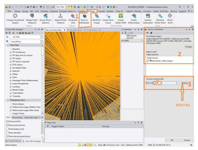
UASMaster will automatically open and all primary settings within the software should automatically be configured. You must now save your project.
