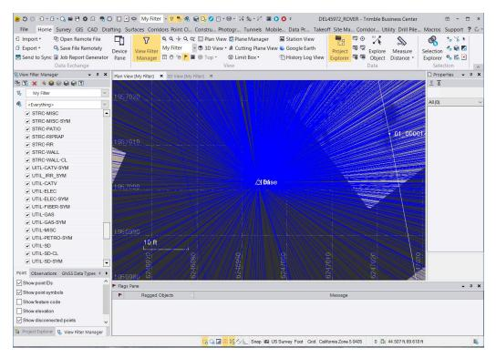
Verify the two base positions are similar by using the **inverse** or **measure distance** command to check the distance and elevation between the two base station points. For this example, points "101" and "base" were used.
