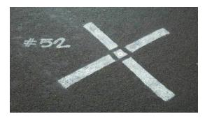
This GCP was spray-painted onto the concrete using a stencil. The marker needs to be large enough to be visible from far away. A center mark helps eliminate any confusion as to where the center point is located.
