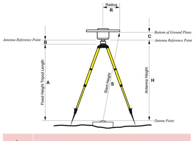
**Pay Attention:** A mismeasured height of the antenna above the mark is one of the most pervasive and frequent mistakes made in GPS control surveying. A best practice is to double measure instrument heights with two different units. (i.e. When operating in the United States, measure heights in both feet and meters.)
